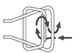
There is a correct way of fixing the straps to a spring anchor. You must ensure the slide bar on the end of the spring is positioned as shown here when looking from above, with the join at the top. Then thread the strap through as the arrow shows.
